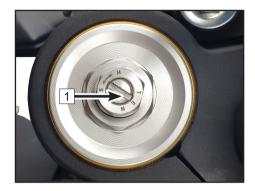
Front shock absorber oil: KHL15 - 10 Front shock absorber volume:365 ± 2mL
